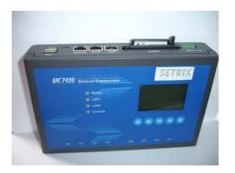
Eight RS-485/RS-232 interfaces are available for connecting the detectors and information displays. Several displays or detectors can be controlled from a single interface via a bus. The basic central control station also has two LAN interfaces. In addition, the system can be connected to the Internet via a LAN and a DSL modem/router.
